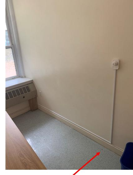
Do not place mini-fridges directly below one of these controls. The heat given off from the fridge will not allow the control to work properly.
